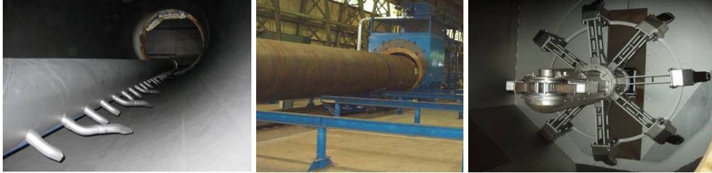
Blast Equipment for Surface Preparation
