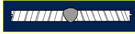
Single Butt-welded Joint, recommended in applications where pressures are in excess of 400 psi
